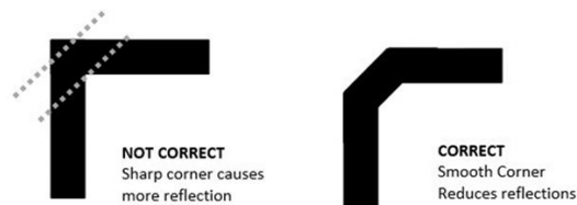
Figure 56. Poor and correct way of bending traces in right angles
